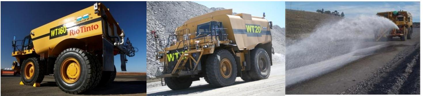
Kador's water tanks can be fitted with the Enviro-spray™ water control system to optimise water usage on mine roads. Conventional water spray control systems have a fixed (or manually operated step variable) water control system which can result in over-watering of mine haul roads when the water truck is travelling slowly or stopped.
