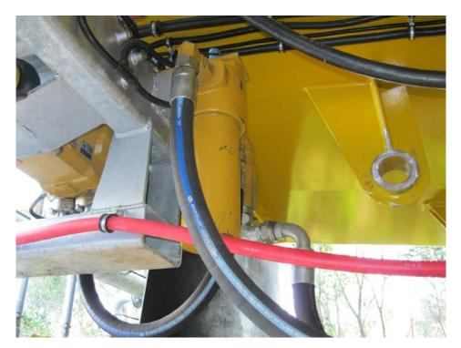
The control of the water volumes is carried out through the standard tilt circuit of the tractor by a control manifold system and a series of dash mounted control switches, the switches are electric over air solenoids to operate the main pump switch, sprays and other options as fitted. The solenoids are mounted in a stainless steel control box at the front of the tank to minimise water ingress. A total pneumatic system is offered as an option.
