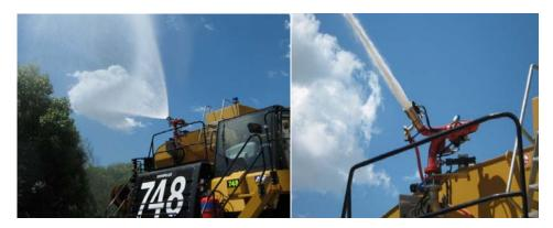
All monitors can be fitted with a foam system also worked remotely from the cab, the foam tanks again are mounted in locations selected by the mines. Stainless steel tanks can be fitted internally or externally to the main tank body, with supply connected to the monitor by a venturi system at a nominate ratio.
