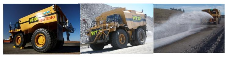
Kador's water tanks can be fitted with the Enviro-spray™ water control system to optimise water usage on mine roads. Conventional water spray control systems have a fixed (or manually operated step variable) water control system which can result in over-watering of mine haul roads when the water truck is travelling slowly or stopped.
