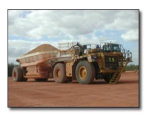
Kador has supplied many bottom dump trailers for coal and bauxite haulage. These can be provided to the client's design, or to Kador's own designs. The fleet of seventeen 195T bottom dump bauxite haulers at a client's mine in Weipa was all supplied by Kador.
